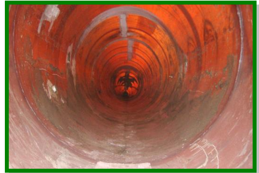
Inside Avatar’s experimental plug-flow digester
